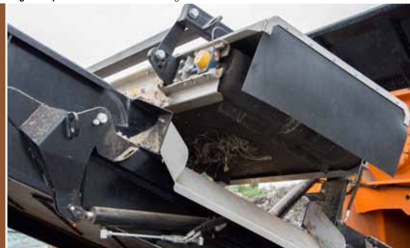
Magnetic separator for extraction of ferromagnetic materials.
