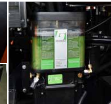
Central lubrication system ensures good greasing of most important parts of the machine
