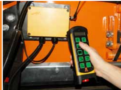
Remote control for basic machine operating functions
