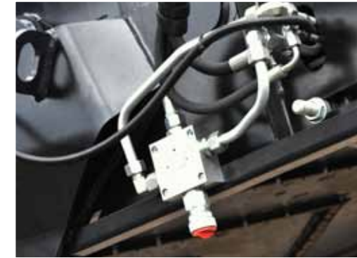
Conveyor belt speed rate adjustment
