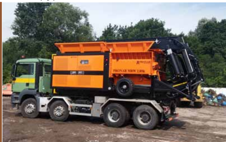
MRW 2.85h - carrying by hooklift frame carriers
