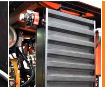
Cleanfix systems automatically clean engine and oil hydraulics radiators
