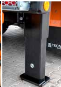
Hydraulic support legs ensures stability of machine
