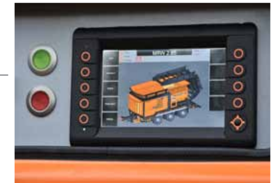
Central control panel with touchscreen
