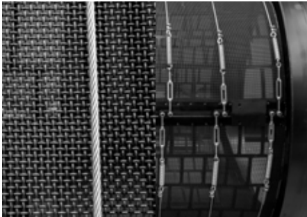
Special mesh drum for perforation <10mm
